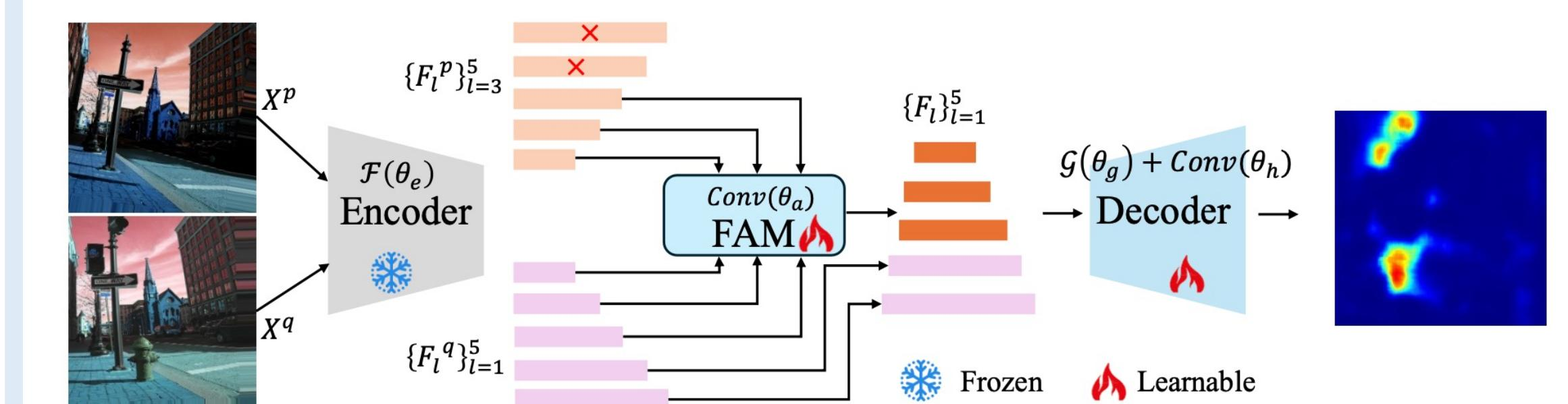
The proposed MetaUAS consists of an encoder, a feature alignment module (FAM), and a decoder. It is trained on a synthesized dataset in a one-prompt meta-learning manner for change segmentation tasks. Once trained, it can segment any anomalies providing only one normal image prompt.
